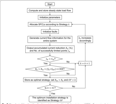
**Fig. 7** Flowchart of the algorithm for determining optimal installation strategy of SFCLs. Parameters being initialized during the third step: number of k = 1; number of installed SFCL  $S_k = 1$ ; maximal current reduction  $R_m = 0$ ; current reduction margin of one additional SFCL= *CRM*; number of measured points  $C_m$ ; optimal strategy OP = 0
