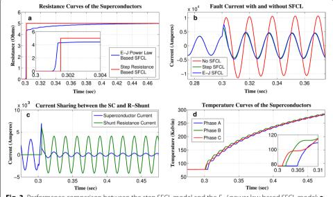
**Fig. 3** Performance comparison between the step SFCL model and the *E–J* power law based SFCL model: **a** resistance growth, **b** fault current characteristics, **c** current distribution in the SFCL, **d** temperature curves of each phase. The displayed insets in subplots **a** and **d** are measured in the corresponding units of the main plot
