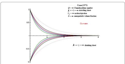
**Fig. 2** Effects of Chandrasekhar number Q on axial  $f_\eta$  velocity in the case of Copper (Cu)-water with  $\phi=0.2$  and  $V_{\rm C}=0.4$
