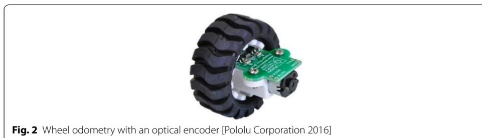
Fig. 2 Wheel odometry with an optical encoder [Pololu Corporation 2016]
