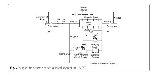
(CTs) are provided at different locations to measure the current for different protection systems. The two Isolators are used to connect the platform and platform equipments to the line or to isolate the platform and platform equipments from the line. The earth switches are used for earthing the platform and platform equipments, as soon as the platform is completely isolated from the line.
