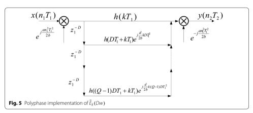
Furthermore, the polyphase implementation structure for decimation and interpolation in LCT domain have many real applications, such as it can perform digital filtering the general case, it also can offer significant saving in computation rate and hardware in two important applications, sampling rate alternation and realization of filter banks.
