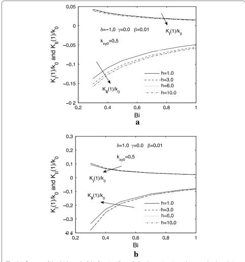
**Fig. 6** Influences of the thickness h of the functionally graded orthotropic strip on the normalized mode l and mode l thermal stress intensity factors, **a**  $\delta = -1.0$ , **b**  $\delta = 1.0$
