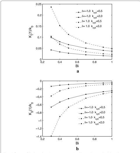
**Fig. 3** Influences of the thermal conductivity parameter  $\delta$  and  $k_{xy0}$  on the normalized thermal stress intensity factors, h=1.0. **a** mode l. **b** mode l
