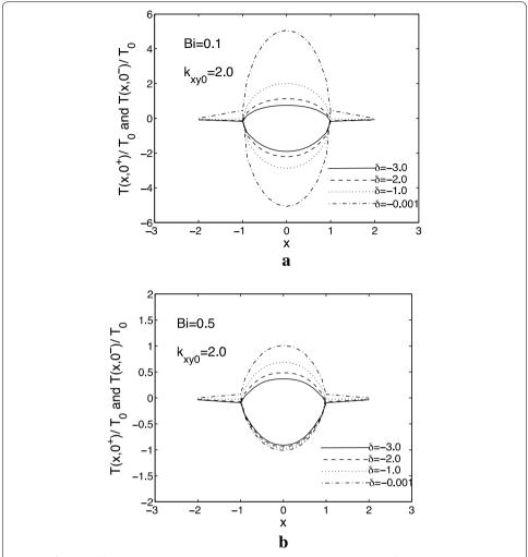
**Fig. 2** Influences of thermal conductivity parameter  $\delta$  on the normalized crack surfaces and crack extend line y=0 temperatures  $T(x,0^+)/T_0$  and  $T(x,0^-)/T_0$ ,  $T_0=Q_0c/k_y^{(2)}$ ,  $t_0=1.0$
