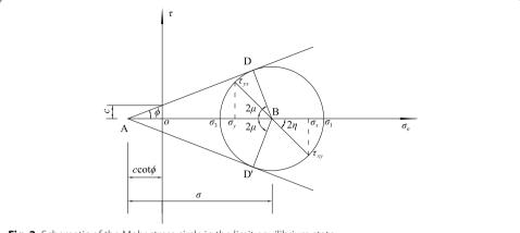
Fig. 2 Schematic of the Mohr stress circle in the limit equilibrium state
