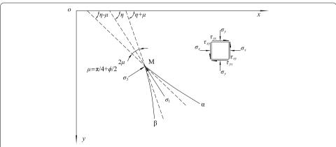
Fig. 1 Notation of soil stress at any point in the limit equilibrium state
