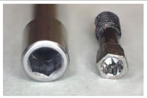
Fig. 2 Abutment screw with head cut into a hexagonal shape
