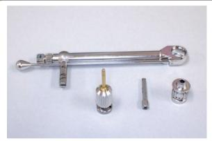
**Fig. 4** Preparation of a torque wrench, hand driver, machined abutment driver, and torque wrench adapter
