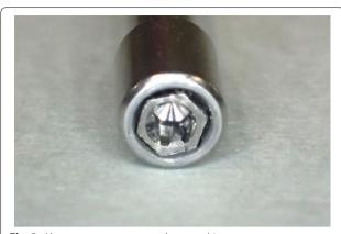
Fig. 3 Abutment screw mounted onto a driver
