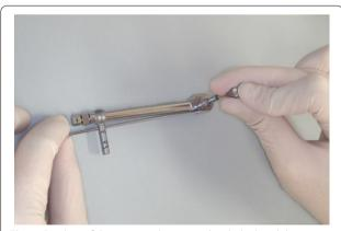
Fig. 5 Reading of the torque value exerted with the hand driver
