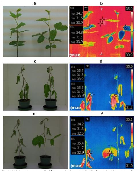
**Fig. 2** Visible (**a, c, e**) and thermal (**b, d, f**) images of soybean plants (Acadian®-treated—*right*, control—*left*), taken by FLIR T-440 camera in environmental chamber Conviron, air temperature 30 °C, relative humidity 60 % on Day 1 (**a, b**), Day 4 (**c, d**) and Day 5 (**e, f**)
