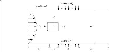
**Fig. 1** Configuration and coordinates (not to scale) for blowing. In the case of suction, velocities normal to the wall are reversed
