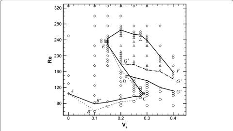
**Fig. 6** Bifurcation diagram in case of suction in the Re  $\sim V_s$  plane: *diamonds*, unsteady flow; *circles*, steady symmetric flow; and *deltas*, steady asymmetric flow
