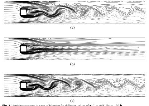
**Fig. 2** Vorticity contours in case of blowing for different values of  $\mathbf{a}V_b = 0.05$ , Re = 175,  $\mathbf{b}V_b = 0.1$ , Re = 175,  $\mathbf{c}V_b = 0.1$ , Re = 250. The *solid* and *dashed curves* indicate positive and negative values, respectively
