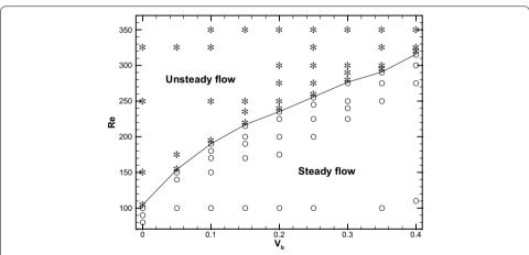
**Fig. 3** The critical curve in case of blowing in the Re  $\sim V_b$  plane separating unsteady and steady flow regimes, based on computed flow states: *stars* unsteady flow and *open circle*, steady flow
