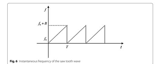
$$f_{if}(t) = f_0 + K(t - nT), \quad nT \le t < (n+1)T, \quad n = 0, 1, 2...,$$
