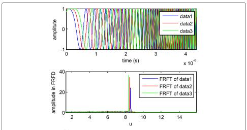
**Fig. 8** Simulation results of the transmitting signal and echo signals (*above*) and their FRFT (*below*) within a modulation period while the target is stationary relative to the detector
