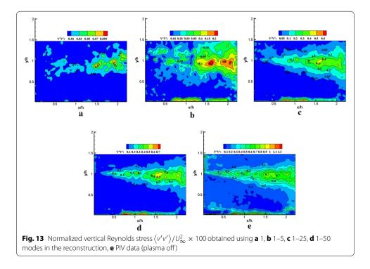
first few lower order modes. The small-scale flow structures appear to be responsible for the recovery of the peak of each Reynolds stress component.
