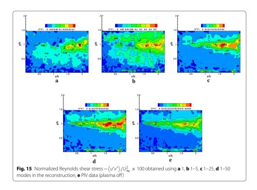
be related to sample size, resolution of the field of view (FOV), and random noise. When using an increasing number of modes in the reconstruction, the streamwise Reynolds stress spatial distribution localized in the narrow strip within the shear layer was gradually recovered. The results indicated that the higher order modes played a crucial role
