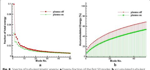
**Fig. 8** Spectra of turbulent kinetic energy: **a** Energy fraction of the first 50 modes, **b** accumulated turbulent kinetic energy  $\sum \lambda\%$
