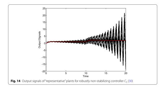
The intentional choice of a controller outside the robust stability region from Fig. 12 evidently leads to the robustly unstable closed control loop. The representative of such robustly non-stabilizing controller is e.g.:
