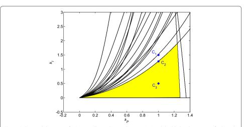
**Fig. 5** Robust stability region for PI controller and interval system (20) with highlighted positions of selected controllers
