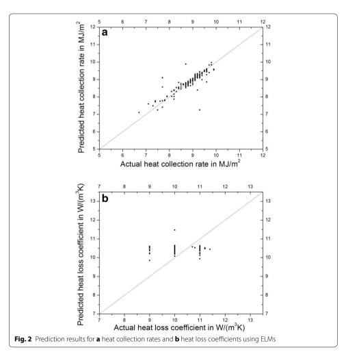
than 10 W/( $m^3K$ ), the deviation belongs to the normal data feature of heat loss coefficients because most of the heat loss coefficients of water-in-glass evacuated tube solar water heaters are around 10 W/( $m^3K$ ).
