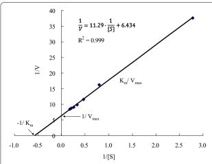
**Fig. 7** Analysis of the enzyme kinetic constants of the recombinant FtsZ. Michaelis–Menten kinetic experiments on GTPase activity of the recombinant FtsZ were performed with final concentration of 1–10 mM GTP as substrate at 50 °C and pH 7.0, and the kinetics  $K_M$  and  $V_{max}$  were calculated
