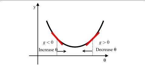
**Fig. 1** Objective value minimization using gradient descent (one variable): if gradient g is positive at  $\theta_k$  then move to  $\theta_{k+1} < \theta_k$ , if gradient g is negative then move to  $\theta_{k+1} > \theta_k$
