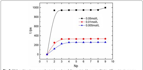
**Fig. 5** DNA melting time versus the total number of disassociated basepairs (Np) in different ionic concentrations (360 K, 11 bp)
