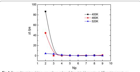
**Fig. 4** The melting interval time versus the number of dissociated basepairs at different temperatures (0.05 mol/L, 11 bp)
