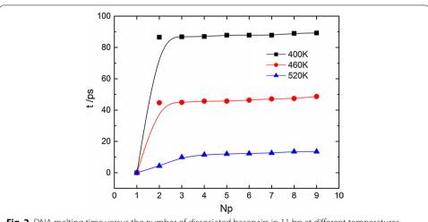
Fig. 2 DNA melting time versus the number of dissociated basepairs in 11 bp at different temperatures (0.05 mol/L)
