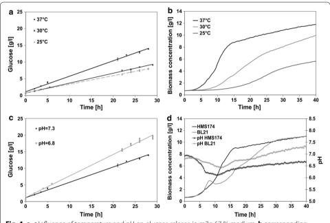
**Fig. 4 a, c** Influence of temperature and pH on glucose release in m2p 67 % medium; **b** corresponding growth of *E. coli* HMS174 at different temperatures and **d** of *E coli* HMS174 and *E coli* BL21 at 37 °C in m2p 67 %. For glucose release and process characteristics, the mean value for triplicates is shown
