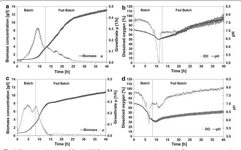
**Fig. 1** BioLector cultivations of *E. coli* HMS174 in enzymatic glucose release media. Biomass course, growth rate (μ), dissolved oxygen (DO) and pH value were analyzed. **a, b** Cultivation with FIT 100 % medium and **c, d** cultivation with FIT 67 % medium. The mean values and the standard errors of the mean for six individual parallel experiments are shown
