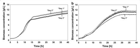
**Fig. 3** Reproducibility of the established small scale fed-batch cultivations: **a** growth of *E. coli* HMS174 and **b** of *E. coli* HMS174(pET11aGFPmut3.1) in m2p 67 %; "Day 1", "Day 2" and "Day 3" are biological replicates of a cultivation performed as sixfold; the mean value and the standard error of the mean for these six individual parallel experiments is shown
