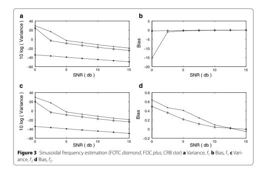
bias for  $f_{m,1}$  or  $f_{m,2}$  is large, which indicates that the estimation is inaccurate below this SNR.
