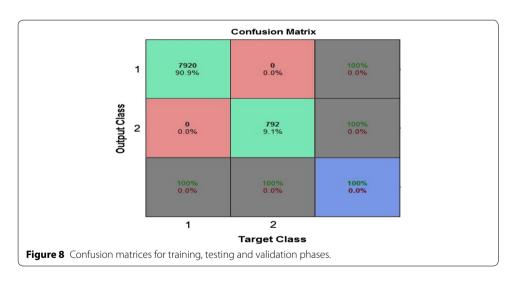
correctly in green and the vice versa in red. It can be seen that the chosen neural network has 100 percent accuracy in fault detection.
