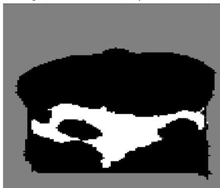
Figure 6 Distinction between black or white fur. Left: Segmented gray scale image of the fur-covered model; Right: The white spot is defined as all pixel with gray scale \geq 25 .
