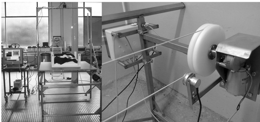
Figure 3 Installation for recording in controlled velocities. Left: Framework with fur-covered model on a wooden plate placed on running rails. SR4K mounted in top view; Right: Motor (background), impeller wheel and rope to tow the wooden plate.
