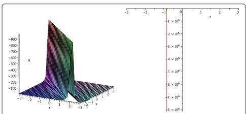
Figure 2 Singular soliton profile of KdV equation for  $\lambda = 3$ ,  $\mu = 1$ , k = 0,  $\alpha = 1$ ,  $\delta = 1$  and wave speed  $\omega = 2$  within the interval  $-3 \le x$ ,  $t \le 3$ . (only shows the shape of  $u_2(\xi)$ ), The left figure shows the 3D plot and the right figure shows the 2D plot for t = 0.
