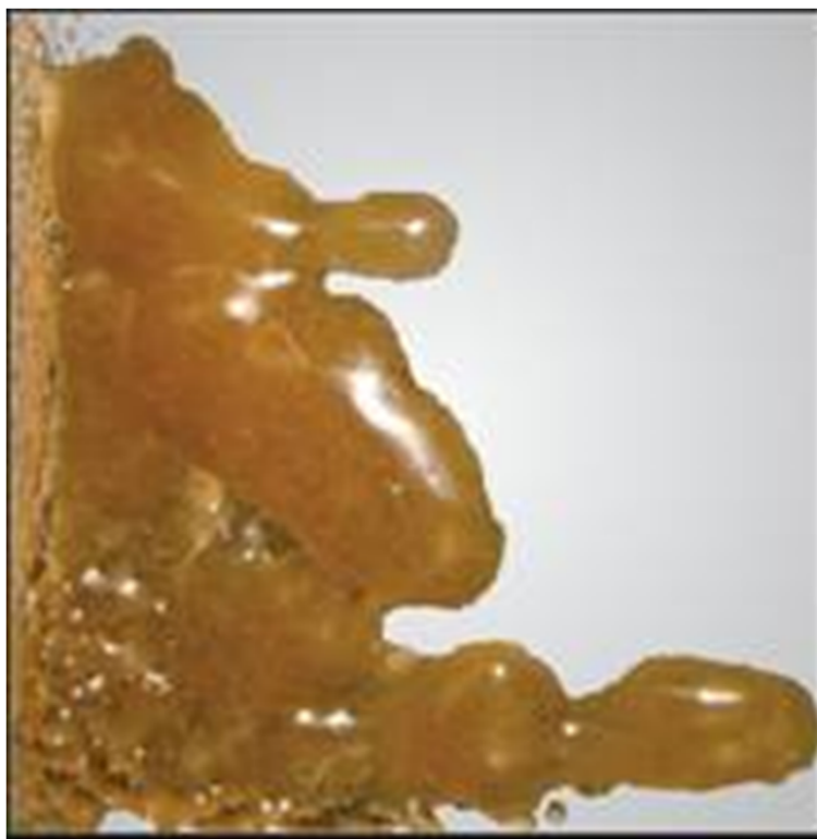
Figure 1 Solid obtained after spray drying autoclaved culture of B. subtilis LBBMA RI4914. Maltodextrin (100 g L -1 ) was added as a drying adjuvant.
