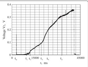
Figure 4 The amplitude value of voltage  $V_2$  across the middle part of the sample as a function of time for  $V_0 = 0.79V$ .
