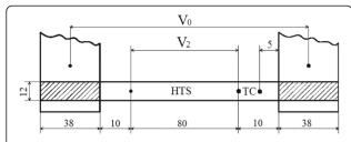
Figure 1 Schematic of the sample with current leads, thermocouple, and probes (distances in mm).
