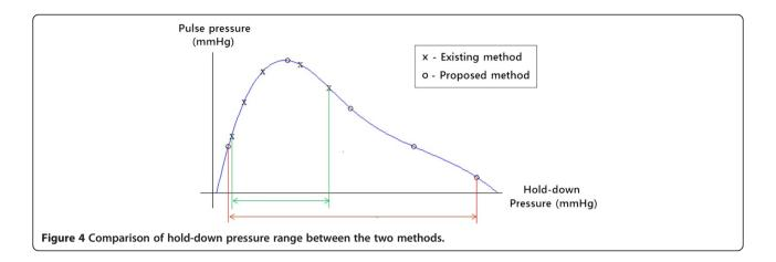
using the measure pulse waves and pulses to compare the two different methods. The pulse depth denotes the motor moving distance from the first pressure step to the last pressure step. To compare the moving distance of the two methods, a paired t-test was performed with a significance level of 0.05. The CFS was calculated by using Equations (1) and (2).
