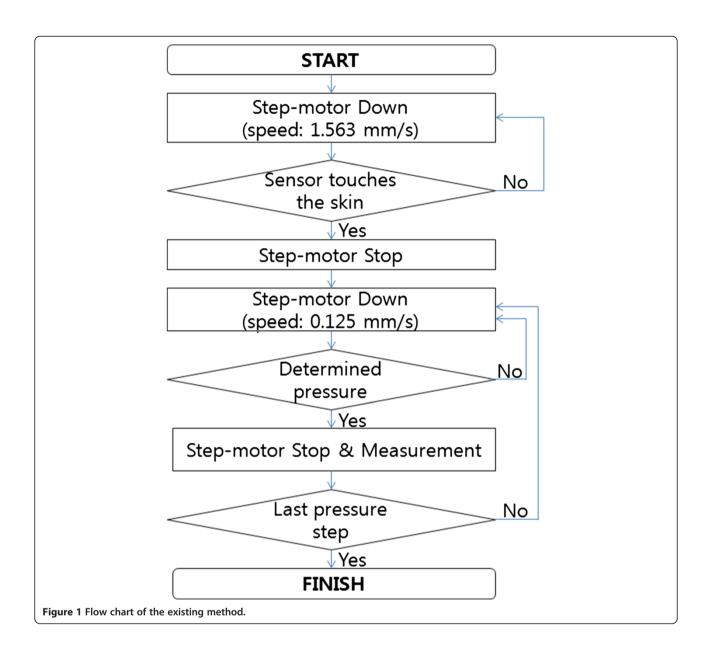
is then determined and divided into five steps. For example, if the hold-down pressures at the first and last points are 25 mmHg and 245 mmHg, respectively, the hold-down pressure at each step is determined as  $1^{\rm st}$  pressure step: 25 mmHg,  $2^{\rm nd}$  pressure step: 80 mmHg,  $3^{\rm rd}$  pressure step: 135 mmHg,  $4^{\rm th}$  pressure step: 190 mmHg, and  $5^{\rm th}$  pressure step: 245 mmHg.
