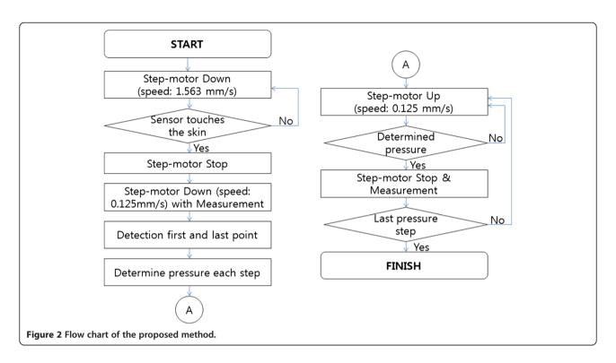
apply appropriate pressure to acquire accurate pulse wave information.
