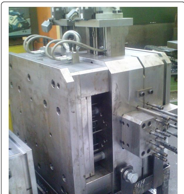
**Figure 5 Die-casting tool—project TL783701.**
