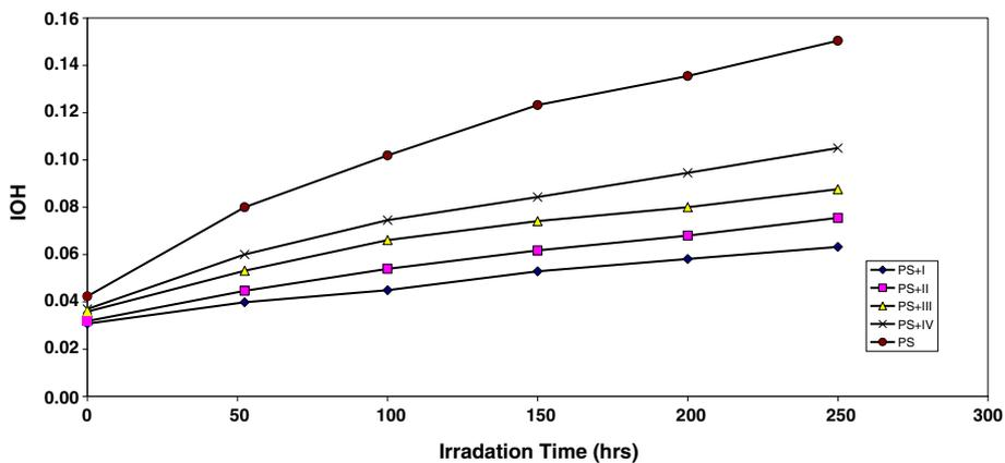
**Figure 2** The relationship between the hydroxyl index and irradiation time for PS films (40  $\mu\text{m}$  thickness). Containing different additives concentration of additives are fixed at 0.5% by weight.
