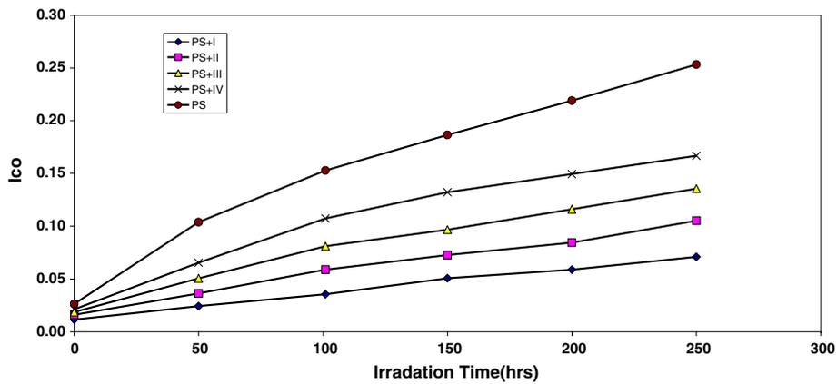
**Figure 1** The relationship between the carbonyl index and irradiation time for PS films (40  $\mu\text{m}$  thickness) containing different additives. Concentration of additives is fixed at 0.5% by weight.
