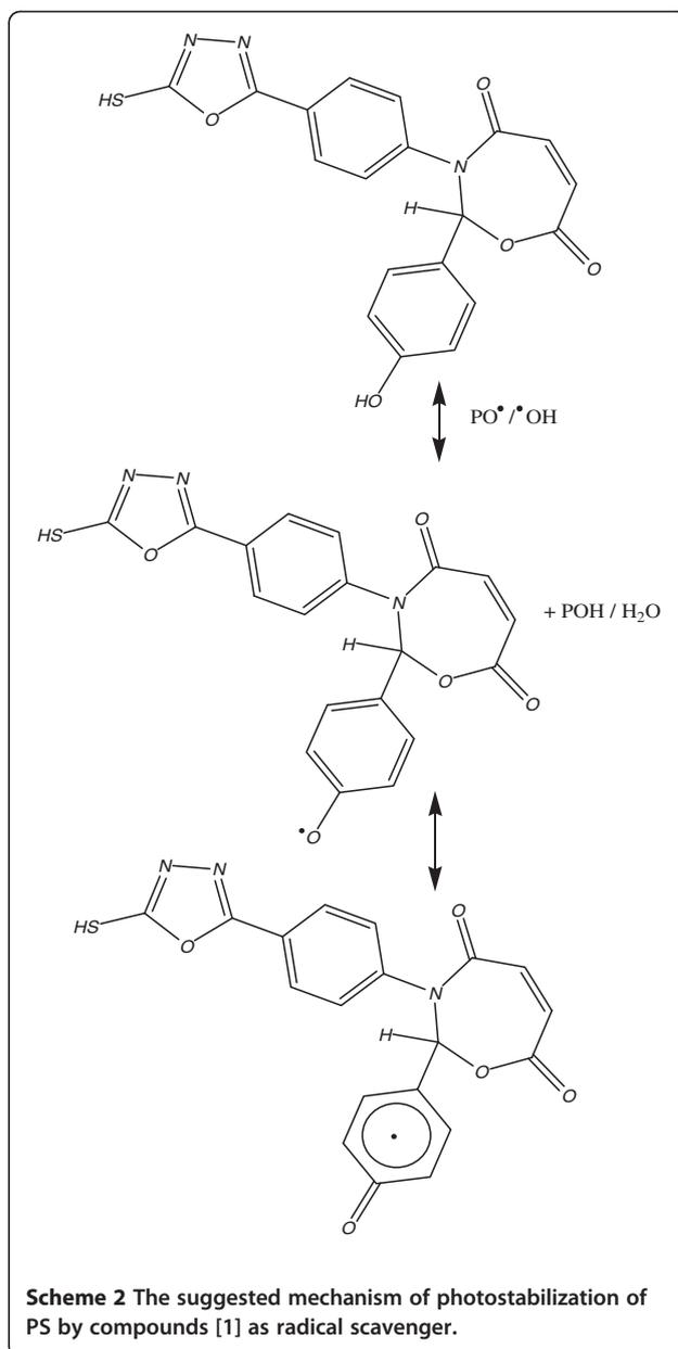
The explanation for low values of  $\Phi_{cs}$  is that in macro-molecule of PS, the energy is absorbed at one site, and then the electronic excitation is distributed over many bonds so that the probability of a single bond breaking is small, or the absorbed energy is dissipated by non reactive processes.
