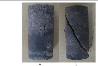
Fig. 5 Failure modes of lime mudstone. a Uniaxial failure. b Triaxial failure
