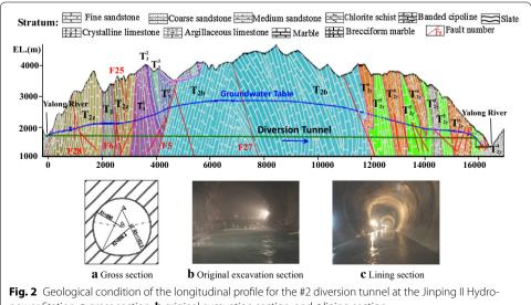
power Station: a gross section; b original excavation section; and c lining section
