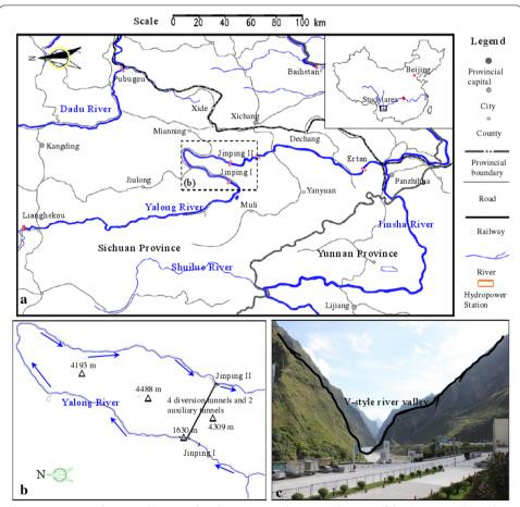
**Fig. 1** Jinping II Hydropower Station and its diversion tunnels group: **a** location of the Jinping I and II Hydropower Stations, **b** layout of the diversion tunnels group and **c** image of the dam site and tunnel intake
