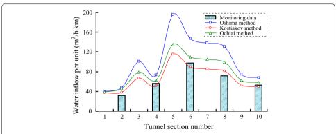
**Fig. 7** Simulated results for the water inflow per unit length using different forecasting methods based on the groundwater dynamics theory
