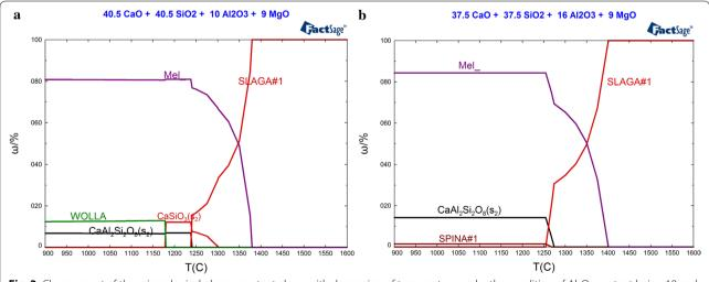
**Fig. 3** Changement of the mineralogical phases content along with decreasing of temperature under the condition of  $Al_2O_3$  content being 10 and 16 %. **a**  $\omega(Al_2O_3) = 10$  %, **b**  $\omega(Al_2O_3) = 16$  %
