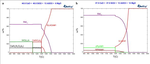
**Fig. 5** Changement of the mineralogical phases content along with decreasing of temperature under the condition of MgO content being 6 and 12 %. **a**  $\omega(MgO) = 6$  %, **b**  $\omega(MgO) = 12$  %
