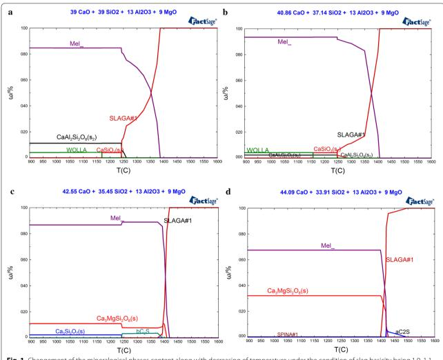
**Fig. 1** Changement of the mineralogical phases content along with decreasing of temperature under the condition of slag basicity being 1.0, 1.1, 1.2 and 1.3, respectively. **a** R = 1.0, **b** R = 1.1, **c** R = 1.2 and **d** R = 1.3
