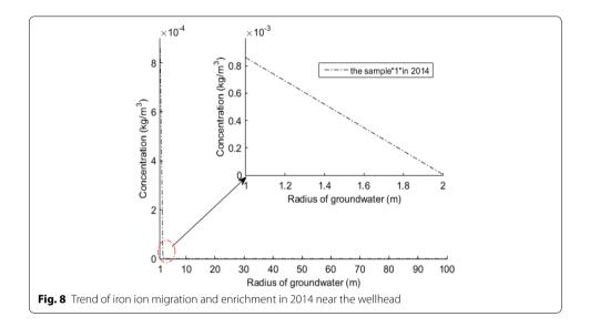
with decreasing radius. The acquired solute concentration and groundwater radius in 2014 is shown in Tables 5 and 6. From this figure, it can be seen that at a radius of 1 m, when  $Q = 432 \text{ m}^3/\text{day}$ , the value has reached 0.86 mg/l, which exceed the standard value of 0.3 mg/l.
