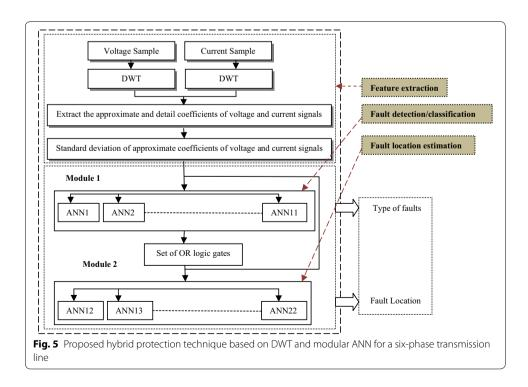
relaying point. Based on the output of first stage i.e. the type of fault, the corresponding ANN of the second stage will be activated.
