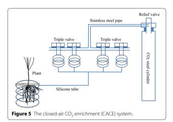
CACE system was much cheaper than the FACE system and convenient in the simulation of below-ground elevated  $CO_2$  in natural conditions.
