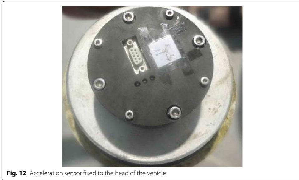
**Fig. 12** Acceleration sensor fixed to the head of the vehicle
