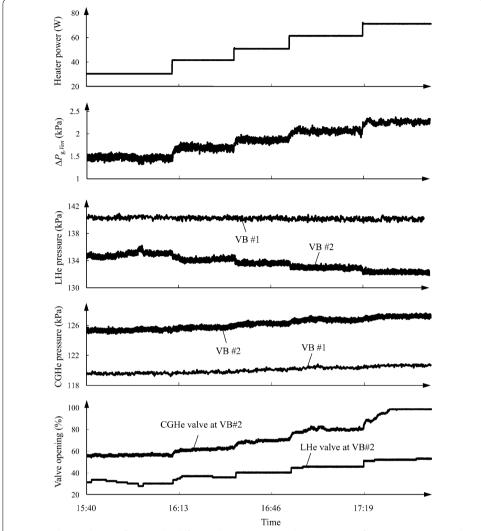
**Fig. 2** Under conditions of case 1, the differential pressure across the Venturi-type flow meter at VB #2 and the CGHe pressures at VB #1 and VB #2 increase when the electric power applied to the heater inside the LHe vessel of S0 is increased, but the LHe pressures at VB #1 and VB #2 decrease. The regulation valves of LHe and CGHe open gradually to compensate for the extra pressure drop caused by increased heater power
