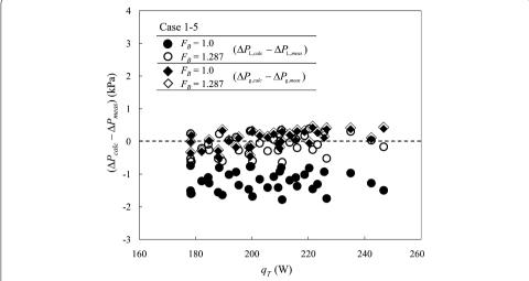
**Fig. 8** For cases 1 to 5 with tolerance factor  $F_B = 1.287$  applied, the calculated total pressure drop for the two-phase LHe supply line approaches the measured results much better, but increases little the results for the CGHe return line
