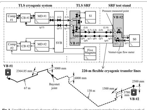
**Fig. 1** Simplified schematic diagram of the cryogenic plants with cryogenic transfer lines and piping path of flexible cryogenic transfer lines of length 220 m to operate the tested SRF module S0 at NSRRC
