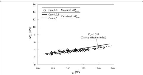
**Fig. 7** The calculated total pressure drop of the 220-m CGHe return line between VB #2 and VB #1 in NSRRC approaches the measured results with tolerance factor  $F_B = 1.287$  applied
