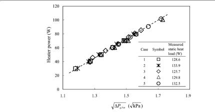
**Fig. 3** The electric power applied to the heater inside the LHe vessel of S0 exhibits a linear dependence on the square root of the measured differential pressure across the Venturi-type flow meter at VB #2. The accumulated static heat load along the LHe supply line is thus derived from a linear fit for these five test cases, i.e. the absolute value of the extrapolating heater power with a zero differential pressure drop read from the Venturi-type flow meter
