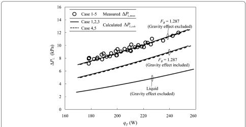
**Fig. 6** With tolerance factor  $F_B = 1.287$  applied, the calculated total pressure drop of the 220-m LHe supply line between VB #1 and VB #2 in NSRRC approaches the measured results much better when the effect of gravity is neglected
