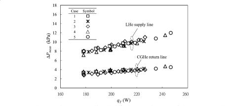
**Fig. 4** Measured pressure drops versus total heat loads for the LHe and CGHe transfer lines; the measured results show that these five test cases can be regarded as one group even though the operating conditions vary substantially
