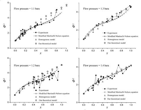
**Fig. 5** Calculated results of two-phase frictional multiplier term  $\Phi^2$  varying with vapor quality  $\times$  with our theoretical model are compared with the experimental data, the modified Martinelli–Nelson equation and the homogenous model (Rane et al. 2011) (Courtesy Cryogenics 2011)
