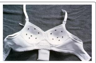
Figure 1 The Chronobra: a custom built thermometric brassiere with 16 channel automated electronic thermometry for measurement of the heat cycle in the breast.
