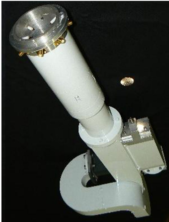
Fig. 4 The newly manufactured GEM 5 GHz OMT. A coin is shown for reference
