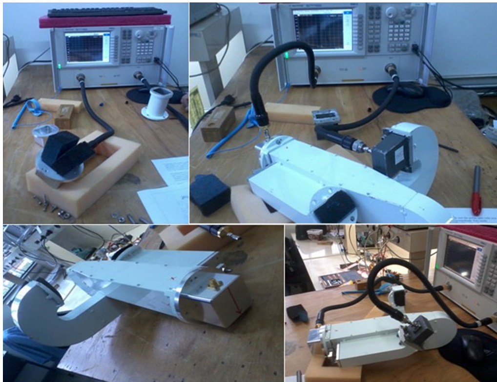
Fig. 6 The measurement setup at the laboratory, showing the network analyzer and the port microwave absorbers
