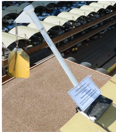
Fig. 3 Flash Flag unit evaluated as a pigeon deterrent on the University of South Africa's Muckleneuk campus
