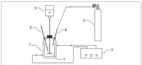
**Fig. 2** Schematic diagram of experimental apparatus for the cooling crystallization of boric acid: *1* crystallizer, *2* thermometer, *3* agitator motor, *4* nitrogen cylinder, *5* thermostat, *6* nitrogen tunnel, *7* impeller
