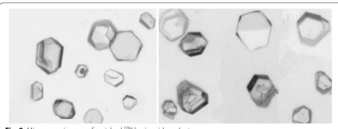
Fig. 9 Microscope images of enriched <sup>10</sup>B boric acid product
