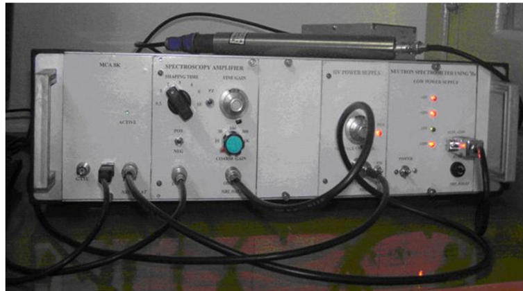
Figure 6 The neutron counting system used at the horizontal channel of the reactor, NRI, Dalat.
